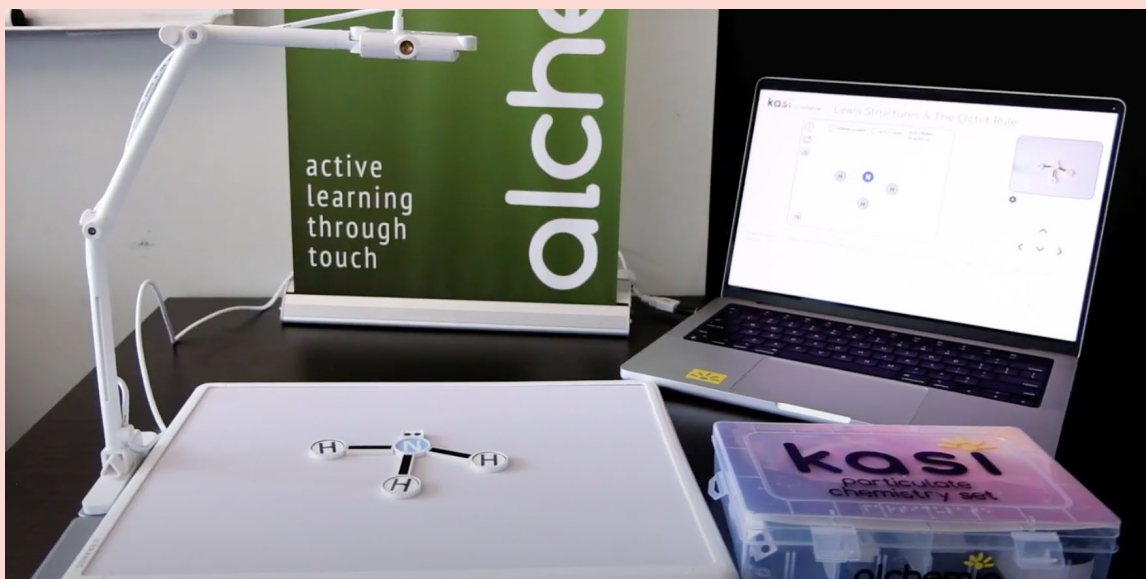
Figure 14. Learners can use manipulatives to create letters on the Kasi platform. A reflector attached to the camera captures the image. Each Kasi piece also has embossed chemical symbols and braille for accessibility.
